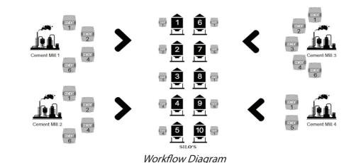
The project includes 4 cement mills, 6 products and 10 different SILOs. Cements can be produced in different mills and go to different SILOs.
